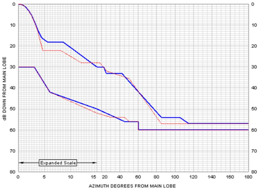
Figure 5: 1ft antenna radiation pattern at 18 Ghz.
