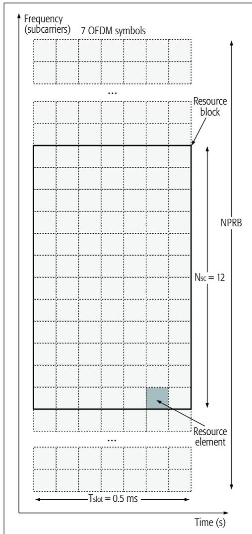
Figure 1. Downlink resource grid defined in LTE.
