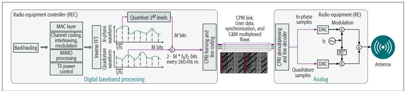
Figure 2. Conceptual explanation of REC/RE functional split.
