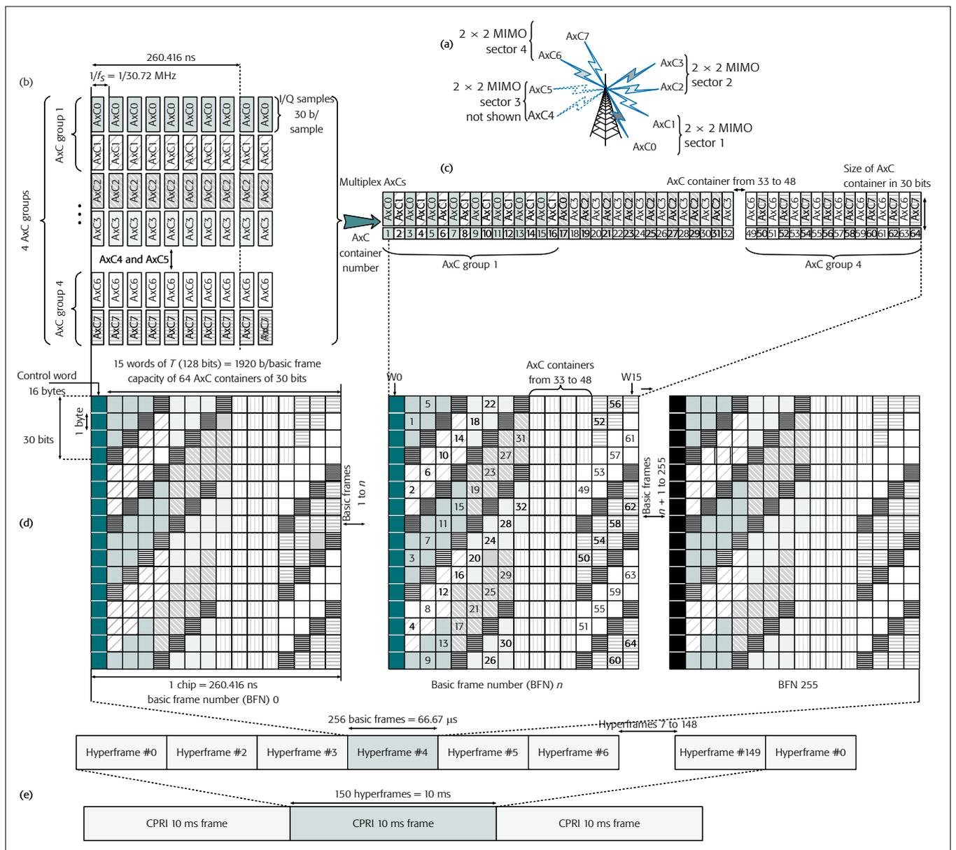
Figure 3. CPRI multiplexing of AxC data in a  $2 \times 2$  MIMO 20 MHz channel use case: a) scenario; b) AxC generation; c) AxC arrangement and serialization; d) basic frame construction; e) hyperframes and 10 ms CPRI frame.
