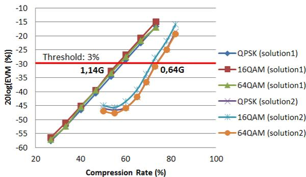
Fig. 4: EVM performance as a function of compression rate
