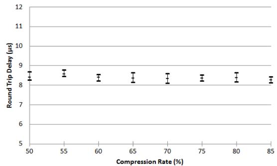
Fig. 5: Round trip delay as a function of compression rate
