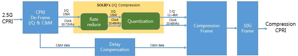
Fig. 2: CPRI compression algorithm
