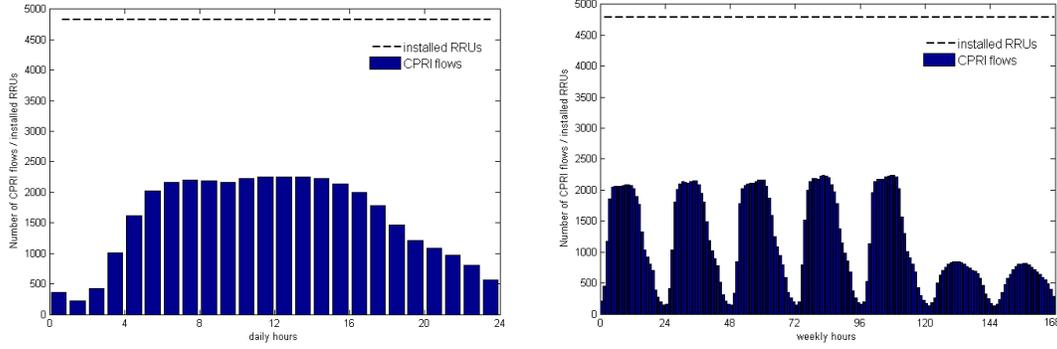
Fig. 2 - Dimensioning values  $n_{CPRI,k}$  as a function of the hour in the cases of daily (left) and weekly (right) traffic profiles.
