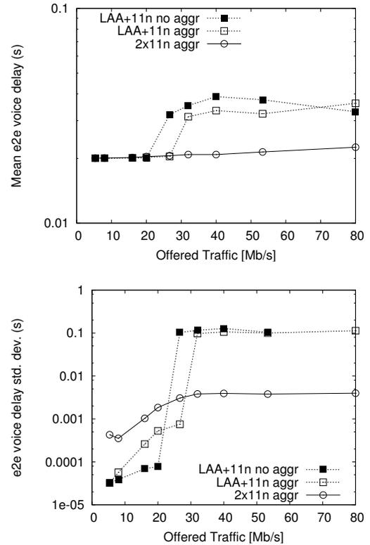
Fig. 9. Comparison among mean end-to-end delay (top) and delay standard deviation (bottom) of VoIP packets in three different network scenarios, as a function of offered traffic; VoIP traffic in *AC\_VO*.
