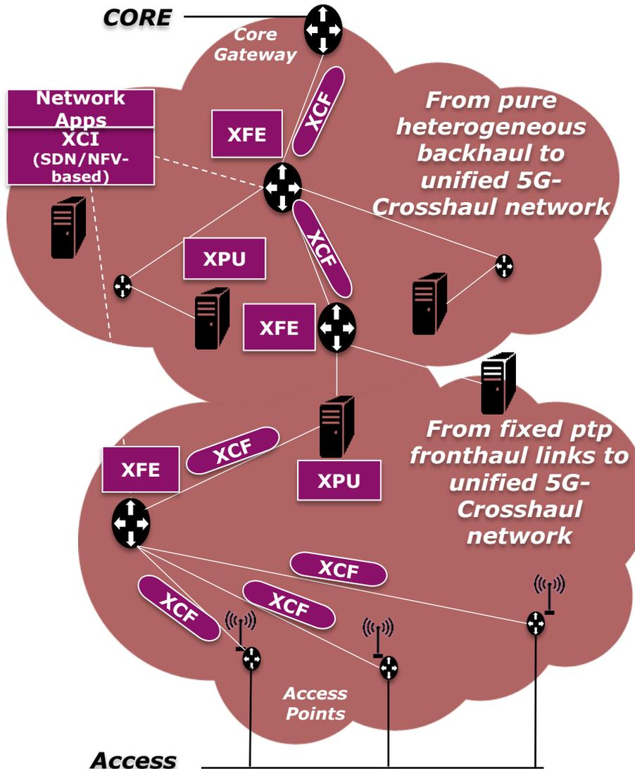
**A holistic approach for converged Fronthaul and Backhaul under common SDN/NFV-based control, capable of supporting new 5G RAN architectures (vRAN) and performance requirements**
